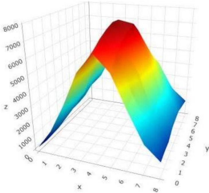
Figure 15: Steel pipe anomaly map in 3D.
